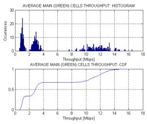
Fig. 4. Histogram and CDF of the DL average cell throughput (SISO)
