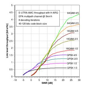
Fig. 2 E-UTRA DL AMC link level throughput with H-ARQ in multipath EPA channel 3km/h
