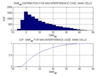
Fig. 3. Histogram and CDF of the SINR perceived by the UEs in the central cells of the scenario.
