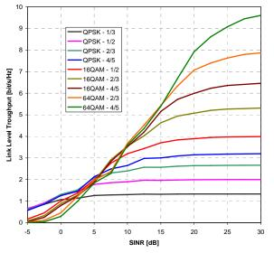
Fig. 7 E-UTRA DL 2x2 MIMO MMSE link level throughput with H-ARQ in multipath EPA channel 3km/h and low antenna correlation
