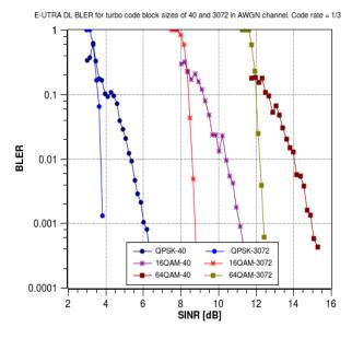
Fig. 2. BLER for two different code block sizes in AWGN channel
