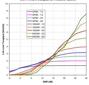
Fig. 8 E-UTRA DL 2x2 MIMO MMSE link level throughput with H-ARQ in multipath EPA channel 3km/h and medium antenna correlation
