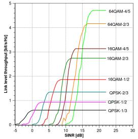
Fig. 3. Mean link throughput vs. mean SINR, for different AMC formats, in AWGN channel and turbo code block size 40-120 bits (no HARQ).
