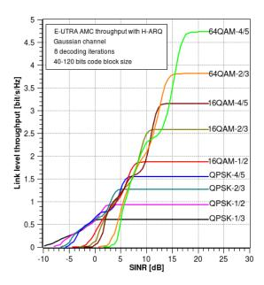
Fig. 4. E-UTRA DL AMC link level throughput with H-ARQ in Gaussian channel (Code block size: 40-120 bits)
