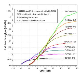
Fig. 6 E-UTRA DL AMC link level throughput with H-ARQ in multipath EPA channel 3km/h
