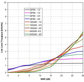
Fig. 9 E-UTRA DL 2x2 MIMO MMSE link level throughput with H-ARQ in multipath EPA channel 3km/h and high antenna correlation
