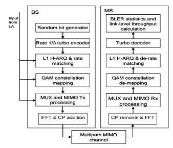
Fig. 1 Block diagram of one MIMO layer of the E-UTRA DL link level simulator
