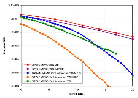
Fig. 2. Uncoded BER vs. mean SIR for different modulations and MIMO configurations in EPA multipath channel @ 3km/h
