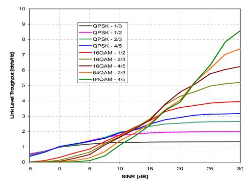
Fig. 3 E-UTRA DL 2x2 MIMO MMSE link level throughput with H-ARQ in multipath EPA channel 3km/h and medium antenna correlation
