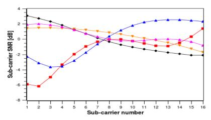
Fig. 6. Several realizations (snapshots) of the ETU multipath channel frequency response showing different frequency selective fading dynamic range. Wideband mean SNR=1dB. Subcarrier spacing=15 kHz
