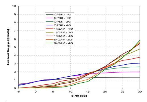
Fig. 4 E-UTRA DL 2x2 MIMO MMSE link level throughput with H-ARQ in multipath EPA channel @ 3km/h and high antenna correlation
