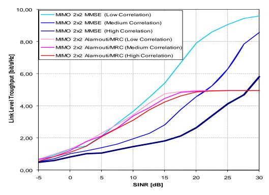
Fig. 5 E-UTRA DL Alamouti vs. spatial multiplexing link level throughput with H-ARQ in multipath EPA channel @ 3km/h
