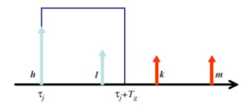
Fig. 4: Detection window in TP j and synchronized with signal h: signals h and l are fully wanted; k and m are fully interfering
