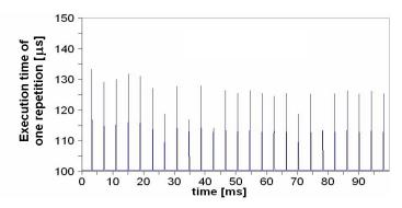
Figure 1: Execution time of the benchmark when run on Strand 0 in Linux
