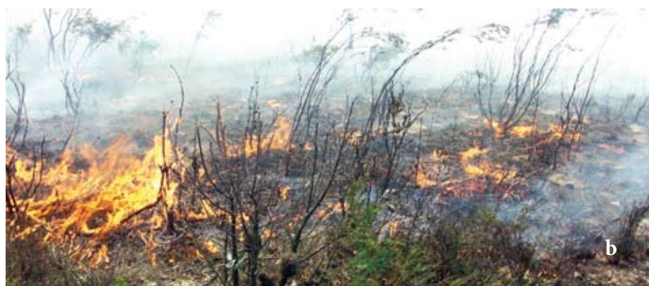
▲ Figure 5: The effect of a direct suppressant drop on fire behaviour as indicated by pre (a) and post drop (b) images taken during the Project FuSE Aerial Suppression experiments. Flames that were up to 2 metres were knocked down to less than half a metre and extinguished in some places. Although this drop had a large influence on this section of fire perimeter, it was not anchored and the fire quickly burnt around it, making it ineffective.
