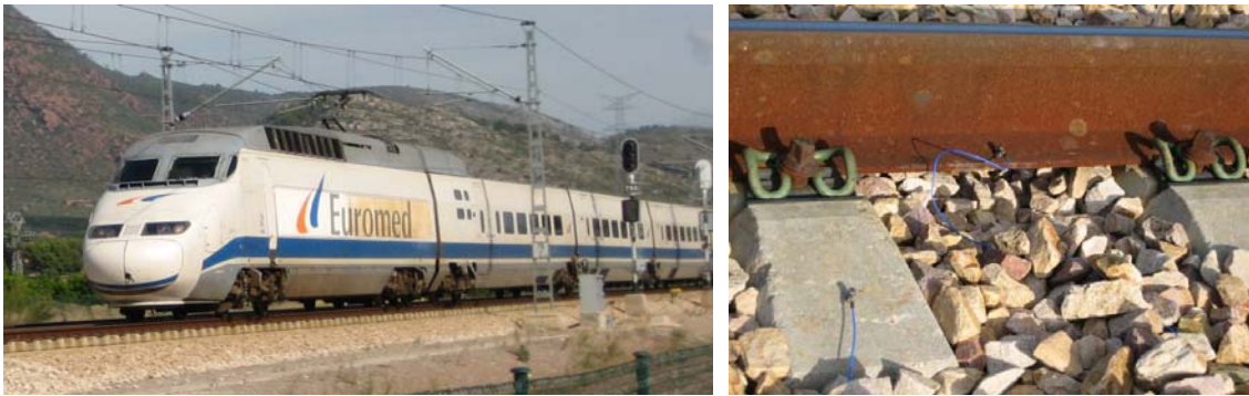
Figure 6: Train pass-by (left hand) and accelerometer locations in rail and sleeper (right hand)
