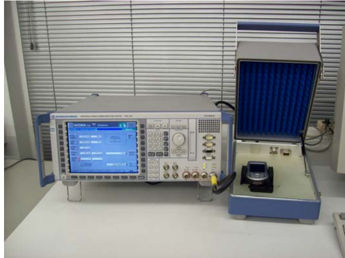
Figure 5. Rohde-Schwarz CMU-200 with 3G mobile to analyze UMTS physical layer parameters
