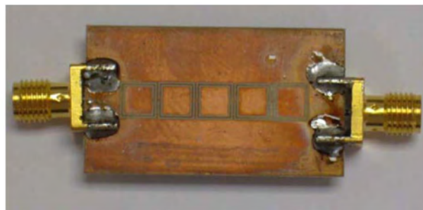
Figure 4. Test prototype of the characterized 5-stage EMI CSRR filter. Dimensions are: host victim line: width=1.18mm, length=35.5mm; CSRRs: a=b=200 \mu m; c=5000 \mu m; 1-stage d=5400 \mu m, 2,3,4-stage d=5200 \mu m; 5-stage d=5000 \mu m.
