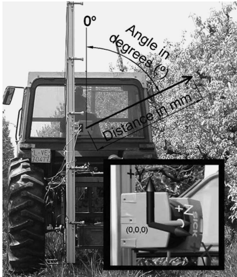
Fig. 2. LIDAR attached to a tractor unit.
