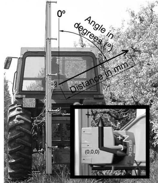
Fig. 2. LIDAR attached to a tractor unit.
