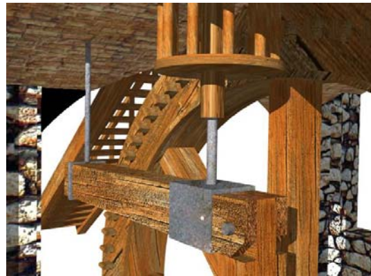
Figure 13. Close-up of the waterwheel and transmission system.
