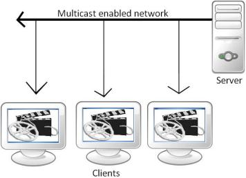
Figure 1: Streaming digital video system.
