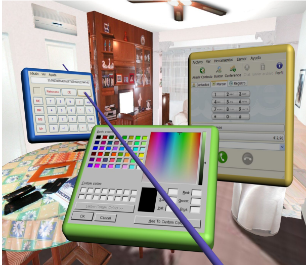
Figure 1: External 2D applications (color selector, calculator and P2P telephony) immersed into a 3D world through a modified VNC client.
