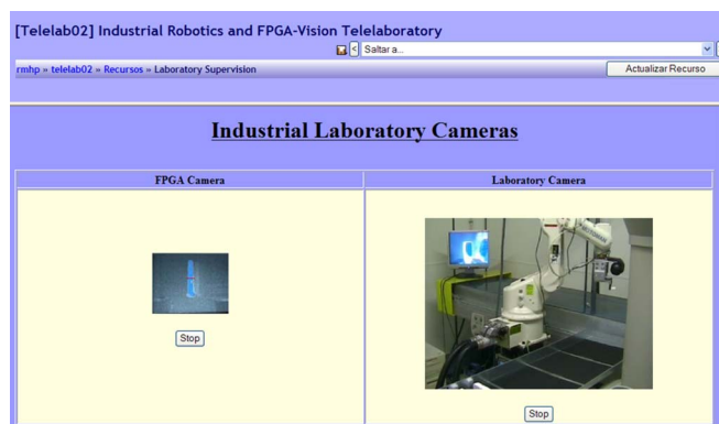
Fig. 2. Web-based interface to the programmable FPGA-vision system (the video on the left represents the output from the FPGA vision system; the video on the right shows the output from a monitoring camera).
