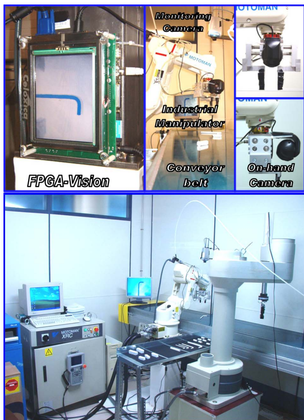
Fig. 1. UJI Industrial Telelab robotics environment (i.e., programmable FPGA-based vision system, conveyor belt, on-hand camera, and monitoring camera from the top).
