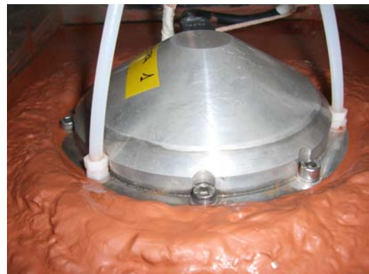
Fig. 5. Coupling of geophone on the sediment.
