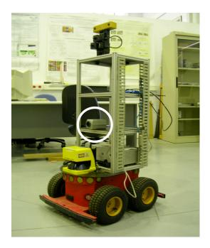
Fig. 3. Pioneer 3AT mobile platform used in the experiments
