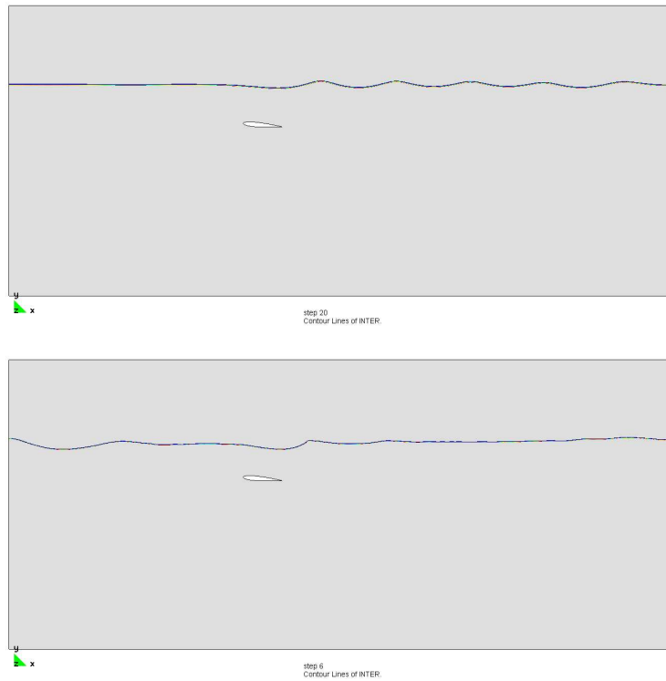
Figure 11: Free surface model at t = 20 (top) and two phase model at t = 6 (bottom), when the solution starts to deteriorate.
