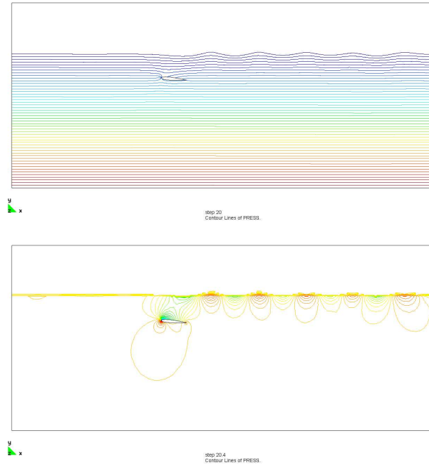
Figure 13: Pressure contours at t = 20 with (top) and without (bottom) hydrostatic component (free surface model).
