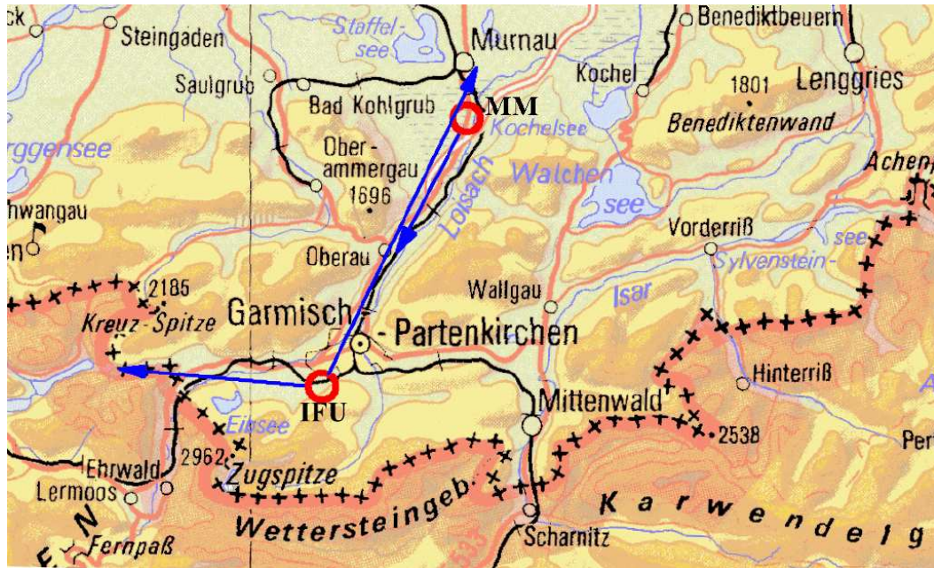
Figure 68: Map of the mountains around Garmisch-Partenkirchen and the Loisach valley; the positions of the two aerosol lidars are marked by circles, the three principal scanning directions by arrows. From the scans along the valleys a two-dimensional map of the backscatter coefficients will be generated.
