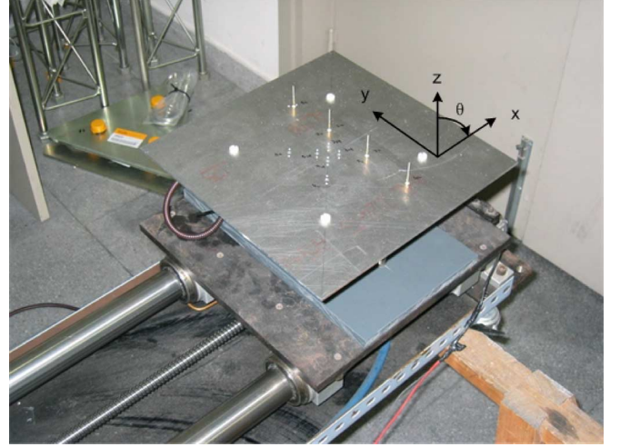
Fig. 1. Picture of the multiomnidirectional-beam MEA consisting of a ULA of omnidirectional monopoles over a finite ground plane, mounted on the automatized measurement setup.
