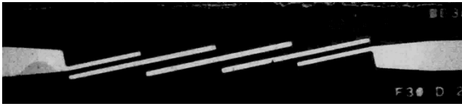
Fig. 11. 30-GHz bandpass filter on Duroid 6002.
