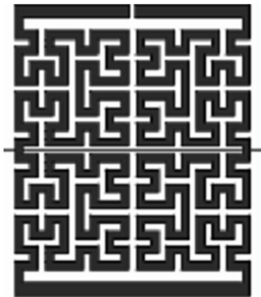
Fig. 6. Hilbert resonator with capacitive load and accessible mid point of folded line (current maximum).
