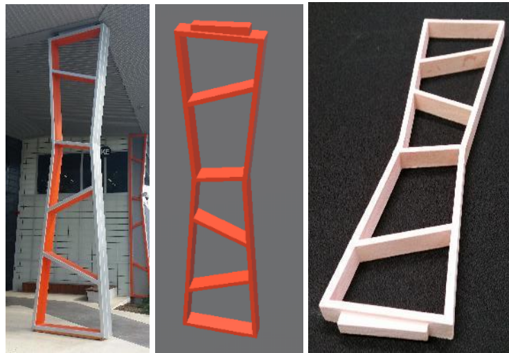
Figure 1: CADET ENTRY COLUMN (I) ACTUAL OBJECT (II) SCREEN GRAB FROM 3D VIEWER (III) PRINTED ITEM.
