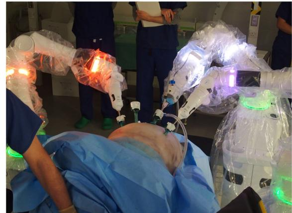
**Fig. 3** Physical arrangement of the new robot-assisted surgical system. Image of the physical arrangement of the new robot-assisted MAS system setup during RALH, corresponding to the left panel shown in Fig. 2b. Visualisation BSU in white and instrument BSUs in orange and green. BSU, bedside unit; MAS, minimal access surgery; RALH, robot-assisted total laparoscopic hysterectomy
