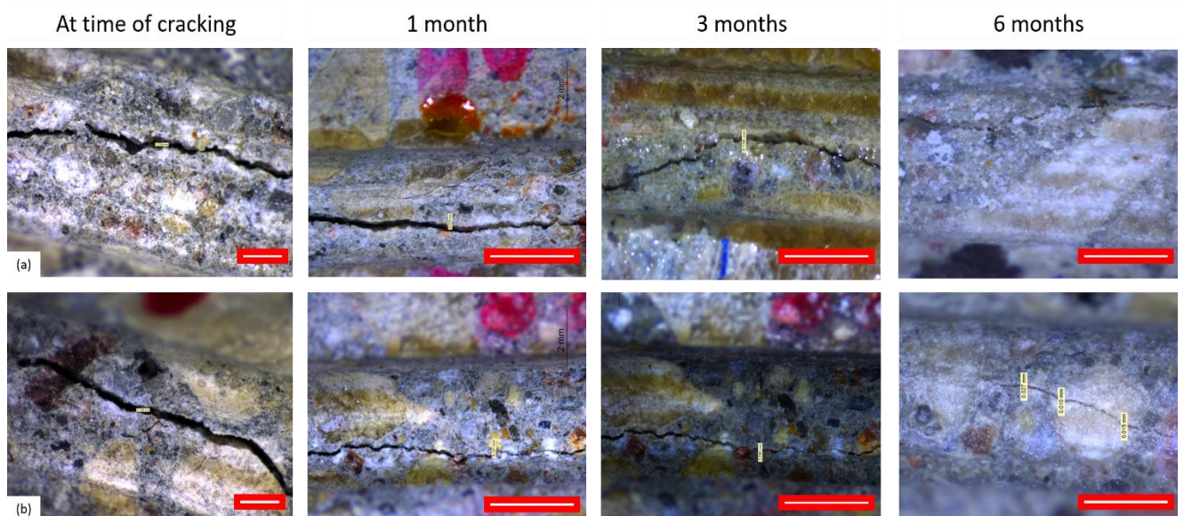
Figure 3. Indicative images of crack healing at time of cracking and at different healing periods for (a) REF and (b) ADD specimen. A gradual reduction of the crack width can be seen with increase of healing period. Yet no precipitation of healing products was observed. (Scale 1mm).
