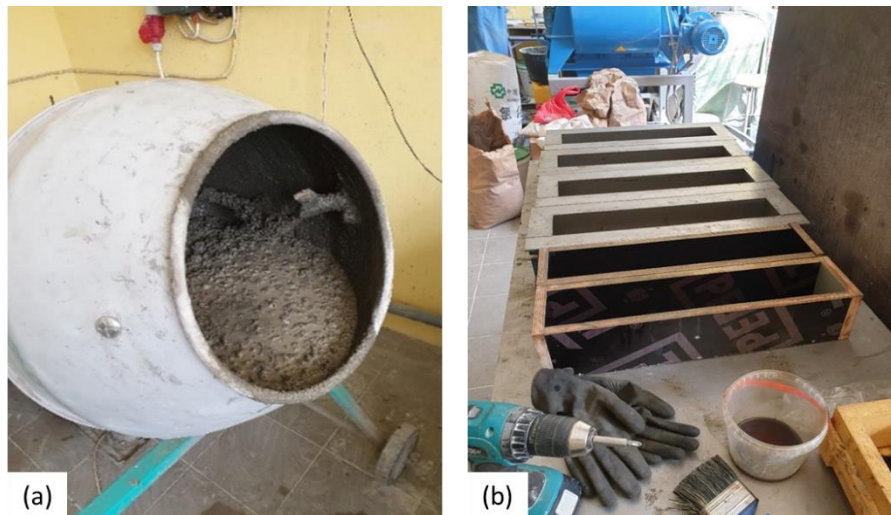
Figure 1. Sample preparation of concrete specimens with mineral additions (a: mixing; b: moulds used for casting).
