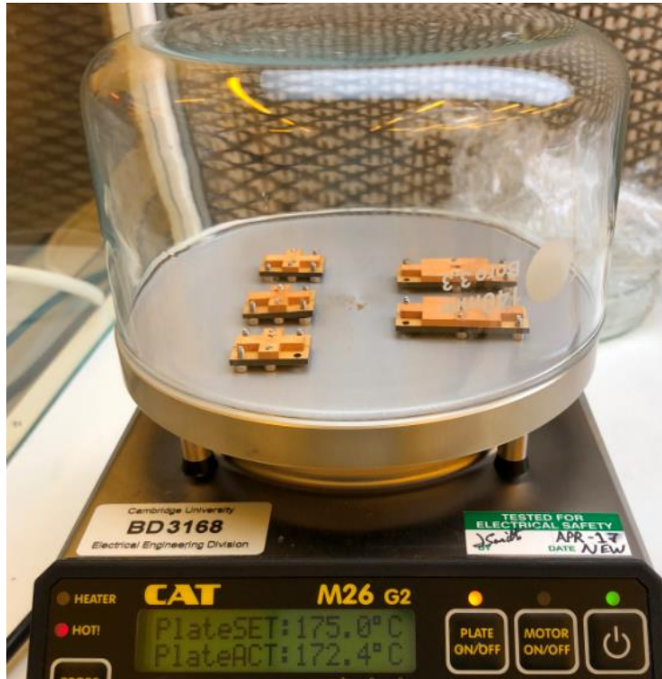
Fig.89 Heating the Assembled Substrates in Preparation for LC-filling
