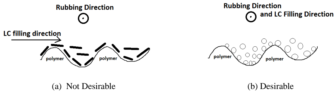
Fig.12 Implications of the LC-Filling Direction and the Rubbing Direction
