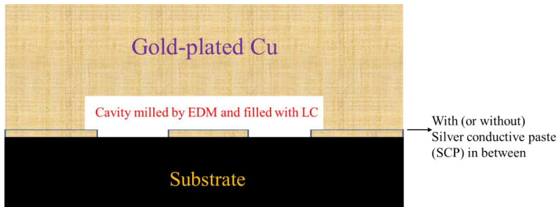
Proposed LC-based Enclosed CPW (ECPW) Structure
