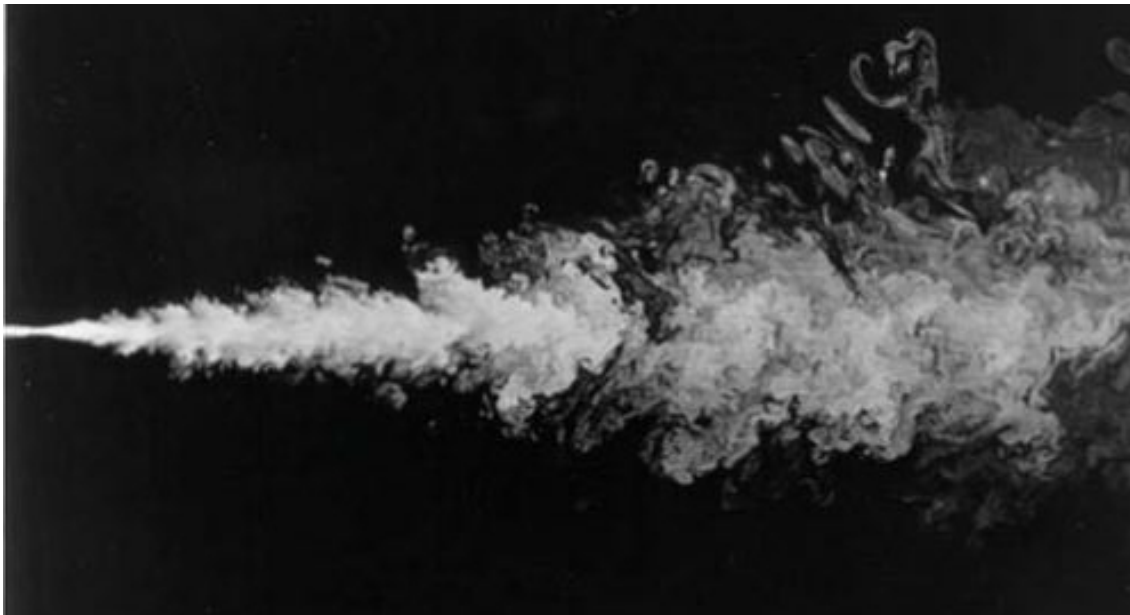
Fig. 1.2: Flow visualisation of a ventilated annular air jet issuing from an open-core slender annular source with D_i/D_o = 0.981 , D_v/D_i = 0.90 and a Reynolds number based on the square-root of the slot area (defined in (1.2)) of Re_f = 35,000 . For details of the nozzle dimensions and design see §2.1. The flow was visualised using a laser on the mid-plane of the jet with vaporised olive oil particles fed directly into the intake of the supply pump (for further information see §2.3).
