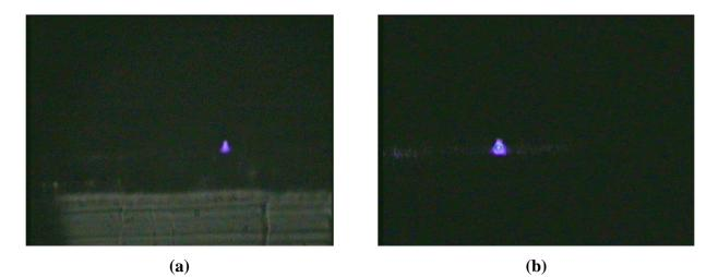
Figure 5.28 – Intensity field profile of (a) 2.5x3 and (b) 3x3 µm siloxane ridge waveguide captured on a CCD camera at 50x magnification
