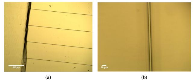
Figure 5.55 – Fabricated high quality siloxane waveguide arrays (2.5-5 µm wide and 3µm high) (b) with microfluidic well (a) formed by the patterned cladding
