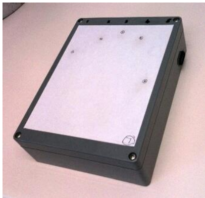
Figure 5.3: Handbox used to deliver soft touch stimuli
