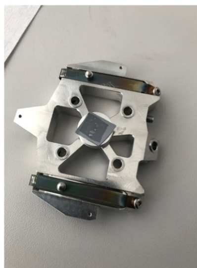
Figure 6.4: Skin sample preparation for SEM-EDX analysis. A: Sample 1 being cryosectioned in a Bright Clinicut cryostat. B: A frozen skin section on a silicon slide being prepared for SEM-EDX analysis.
