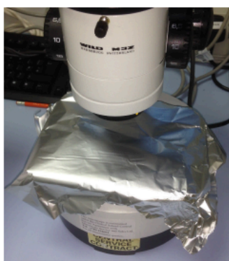
Gelatine samples were halved under microscope over aluminium foil wrapped around dry ice.
