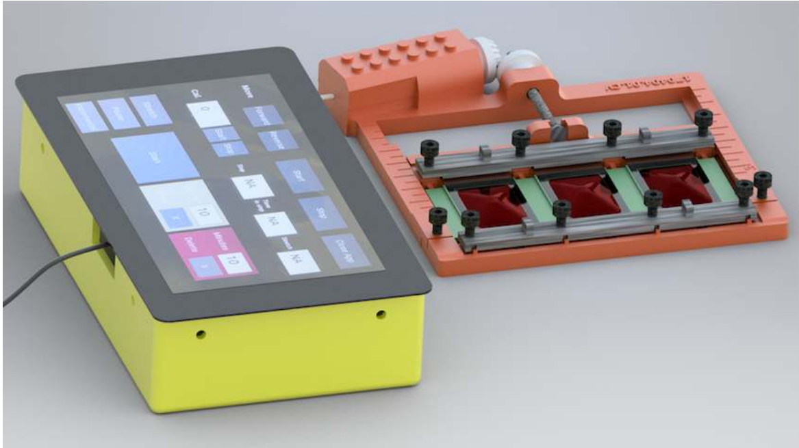
Figure 4.5 Set-up of the automated stretcher. The motor is connected to a Raspberry Pi (yellow box) and touchscreen that allow the user to control the protocol.
