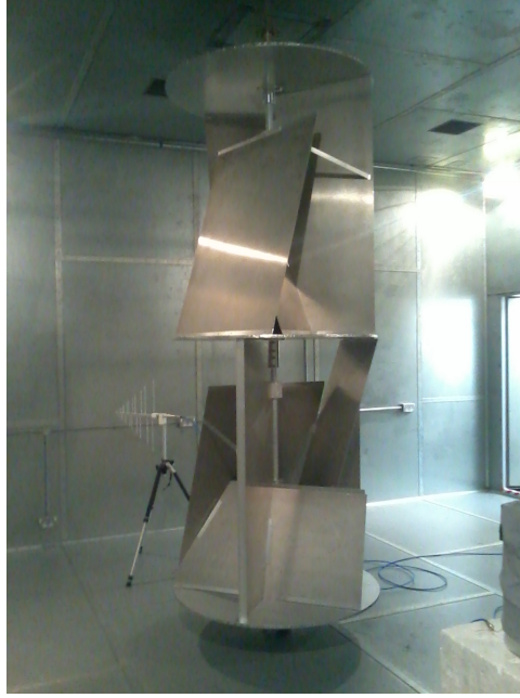
Figure 2.1: Stirrer in the National Physical Laboratory reverberation chamber
