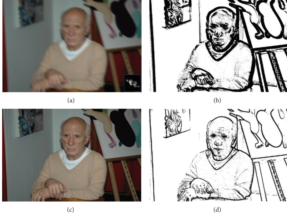
FIGURE 2: Reference map estimation. (a) Input blurred image. (b) First reference map is estimated from the blurred image. It can locally compute smooth regions and distinguish different edge regions. (c) The deconvolved image with the first adaptive regularization. (d) Second reference map is estimated from previous deconvolved result.
