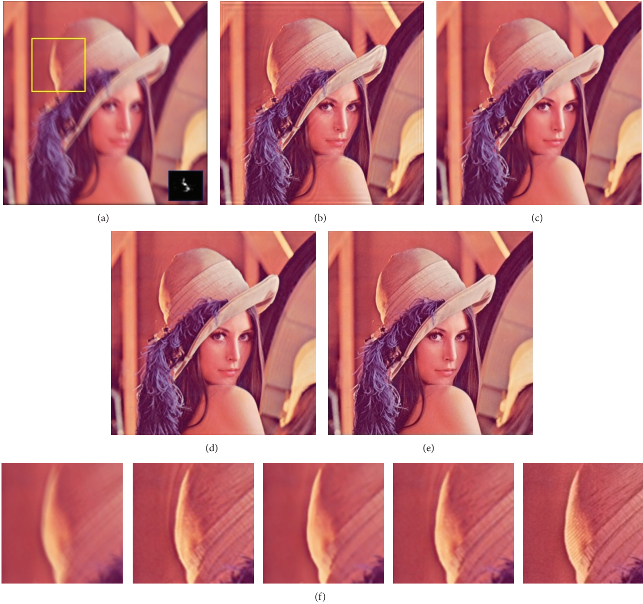
FIGURE 4: Deblurring results of synthetic photo “Lena.” (a) The size of blurred image is 512 \times 512 , and the estimated PSF size is 33 \times 39 . (b) The standard Richardson-Lucy method. (c) The result of Levin’s method [5] with the sparse prior. (d) The result of Krishnan’s method [7] with the hyper-Laplacian prior. (e) The result of our deconvolution with adaptive regularization. (f) Close-ups of (a)–(e) image regions for comparison.
