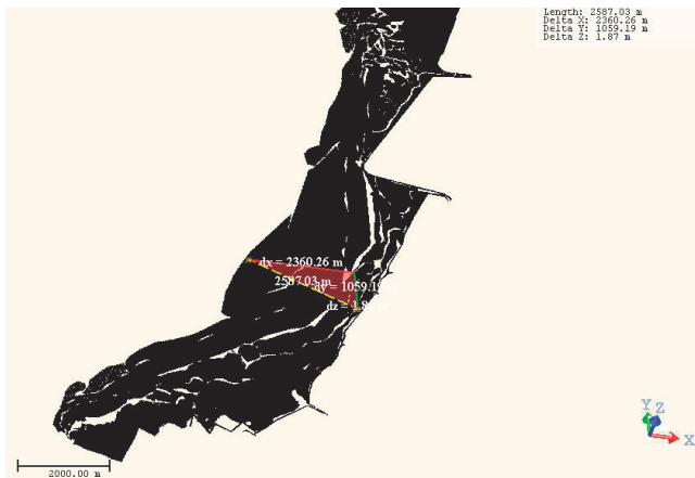
Fig.6 Cloud point data results collected from the coast line with the furthest scan distance from the coast line at 2,587m
