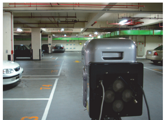
Fig.3 Three-dimensional laser scanner erected 30m away
