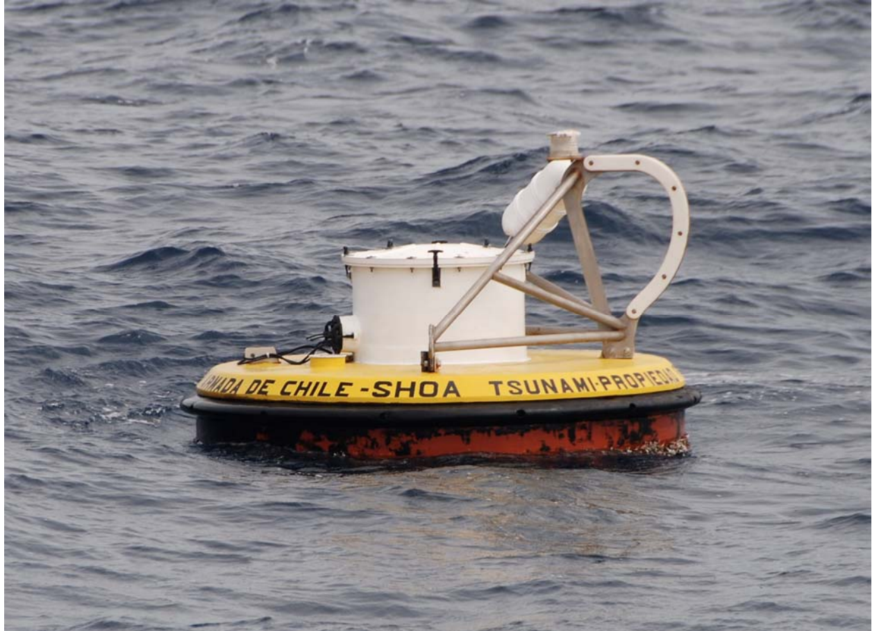
Figure 5-12. DART II surface mooring inspected during Stratus 11 cruise.
