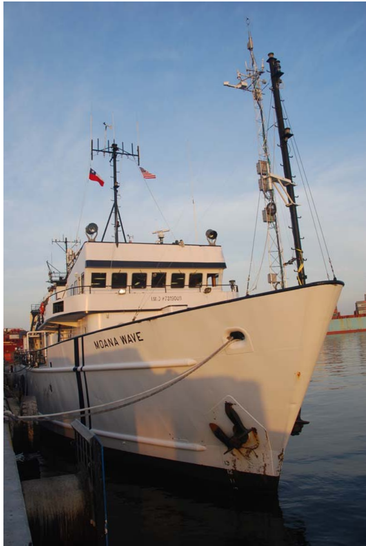
Figure 3-12. Picture of Moana Wave . Meteorological ESRL tower is installed behind the bow mast, on O1 deck. Sonic wind is installed on bow mast and VOS sensors are on top of the wheelhouse.
