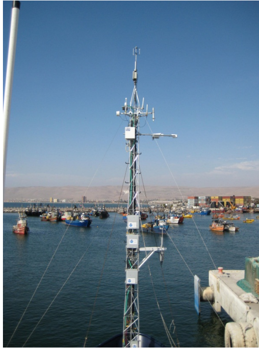
Figure 3-8. Turbulence Flux system setup on the tower in behind the jack staff of the R/V Moana Wave . WHOI turbulent anemometer is at lowest level.
