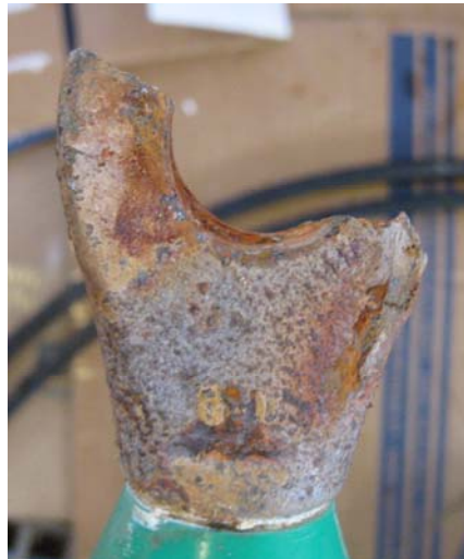
Figure 4-1. Stratus 10 mooring failed part, which was just below the 45 meter SBE 37 on a Ti load bar.
