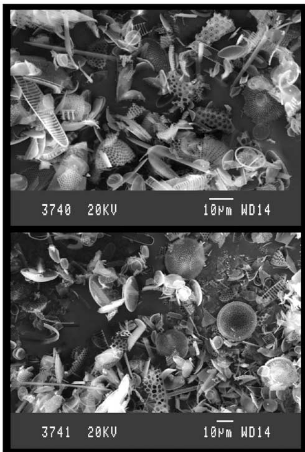
Figure 2. Scanning electron microscope images of separated and cleaned diatom opal from box-core material. The opal is separated from the sediments using a heavy liquid flotation, rinsed thoroughly, then cleaned using a series of reductive and oxidative cleaning steps. Scale bar shows 10 \mu\text{m} .
