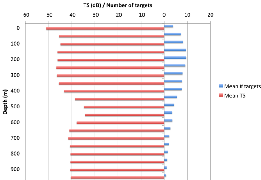
Figure 3. The mean number of targets, target size, and mean scattering volume with depth for the entire study area. There was a peak in 9 targets/2500 m 2 at 200–250 m, a peak in target size of –35 dB at 550–600 m, and a peak in mean scattering volume at 500 m. doi:10.1371/journal.pone.0019269.g003
