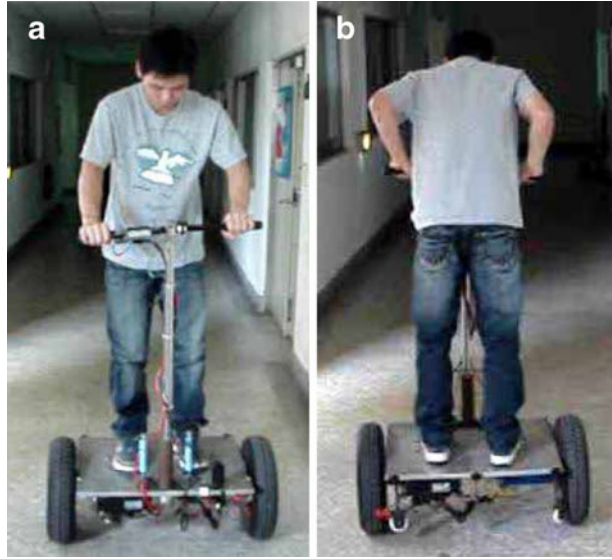
Fig. 12 The moving HTV ridden by the second rider (165 cm/60 kg): a moving forward; b moving backward
