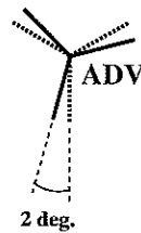
Figure 8.8: Installation errors that are corrected in estimating w_{Earth} in AUV Mission B9804107.
