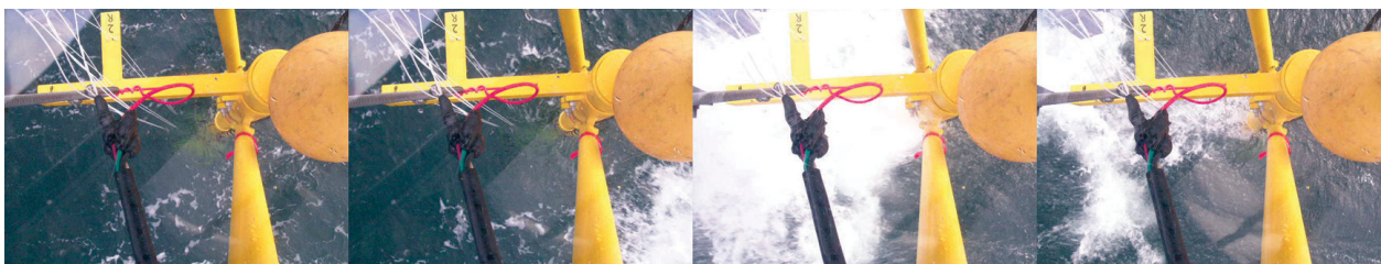
FIG. 16. A sequence of images from the still camera on the spar buoy; images are obtained at 0.4-s intervals. The breaking wave in Fig. 15 can be seen in the last two images.
