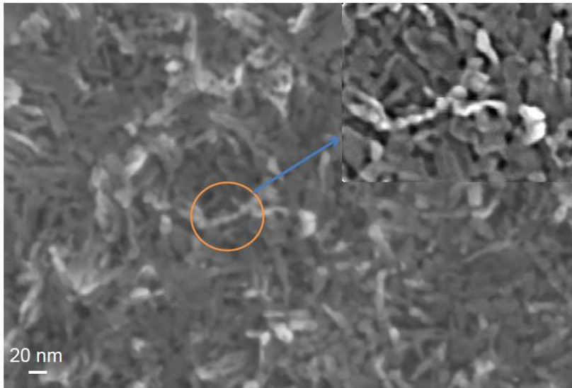
Figure S6. FESEM of chain network photoanode. The inset image shows one of the pearl-necklace chains
