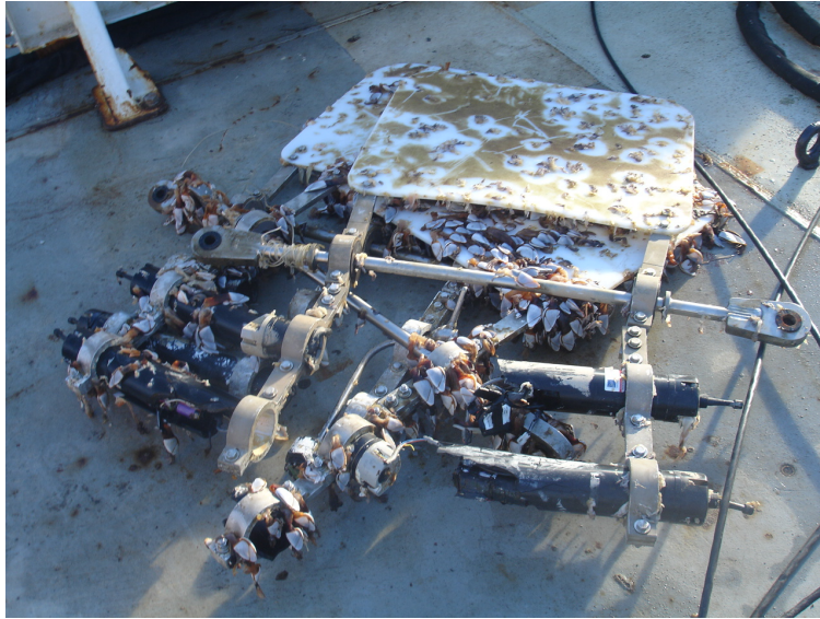
Figure 4-3c. Nortek AS ADCM recovered.
