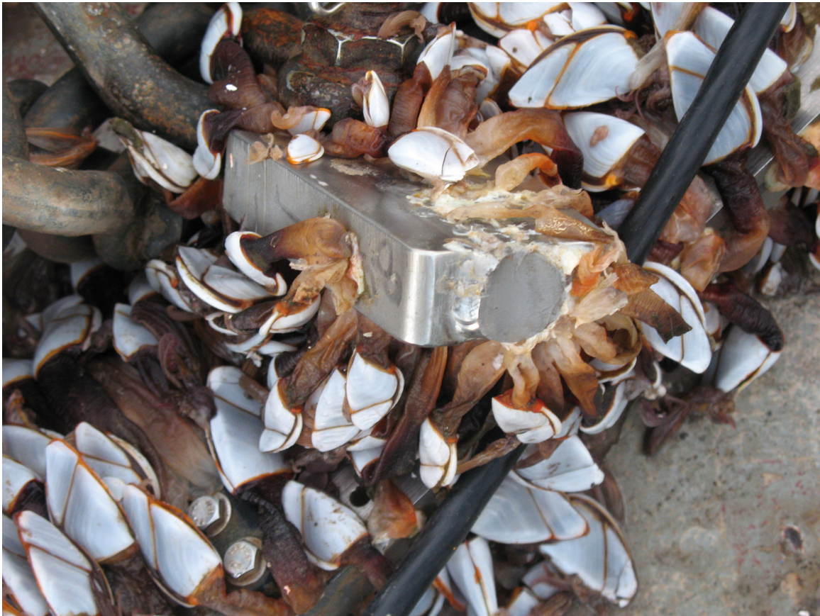
Figure 4-2. Broken titanium alloy load bar at lower end of load bar on the 8.4 m dual Nortek instruments.
