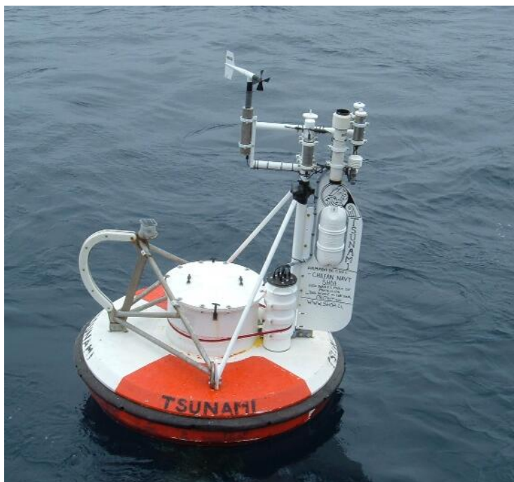
Figure 5-23: DART II surface mooring with a complete set of IMET sensors.
