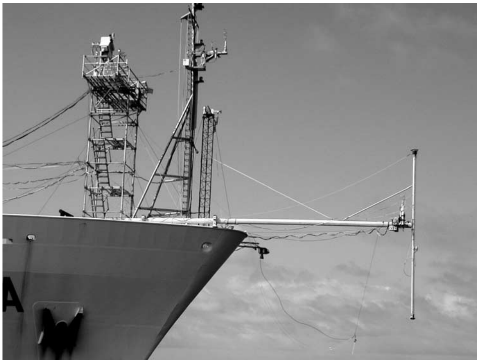
Figure 3. The experiment setup used during the GasEx experiment aboard the R/V Ronald Brown . The mast extended 10 m forward of the bow at its closest point. The figure also shows the flux package deployed by National Oceanic and Atmospheric Administration Environmental Technology Laboratory on the forward jackstaff and the infrared imagery system deployed by University of Washington Applied Physics Laboratory on the scaffolding.
