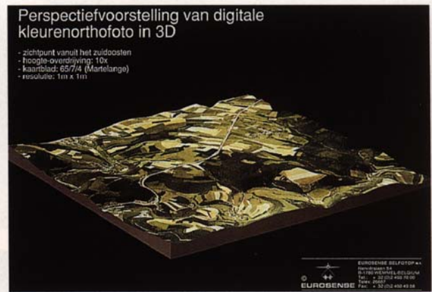
1.4 Digital orthophoto draped over a digital elevation model to provide a perspective view of the landscape
