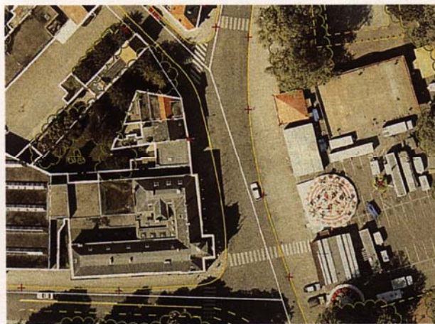
1.5 Large-scale digital orthophoto of urban scene including overlaid vector data on roads and building outlines for a utilities database
