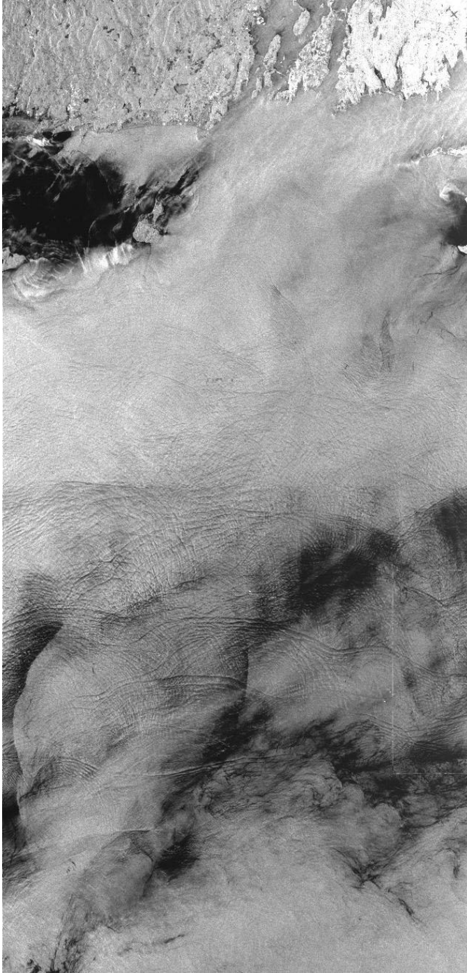
Figure 2. SAR image of the New England shelf on August 8, 1996 shows the surface signature of internal solitons propagating shoreward from the continental shelfbreak. (ERS-2, C-Band, VV) ©ESA 1996.
