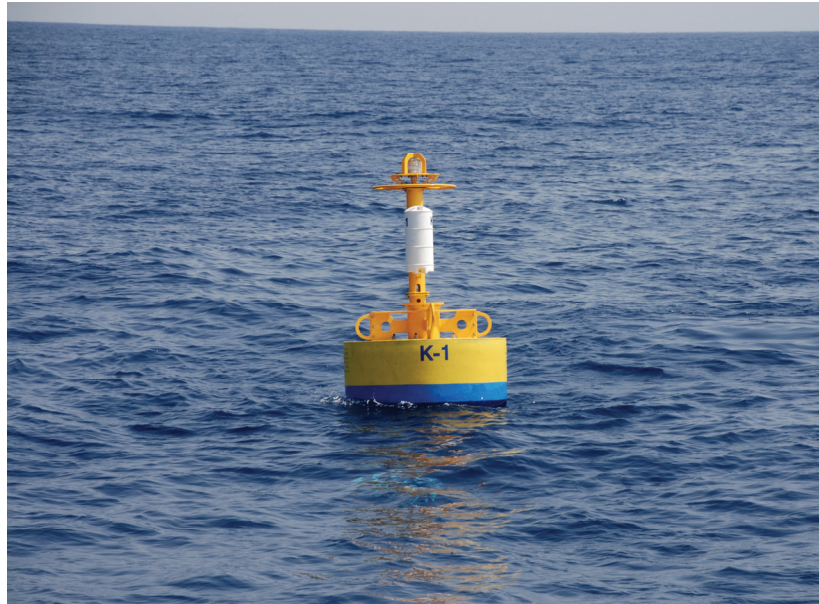
Figure IV-3. Two views of the surface buoy supporting mooring K1. The upper photograph shows the K1 buoy on deck (with the K2 buoy in the background). The white cylinder attached to the underside of the buoy is a Microcat CTD. The lower photograph shows the K1 buoy shortly after deployment (photos courtesy of Susan Avery).
