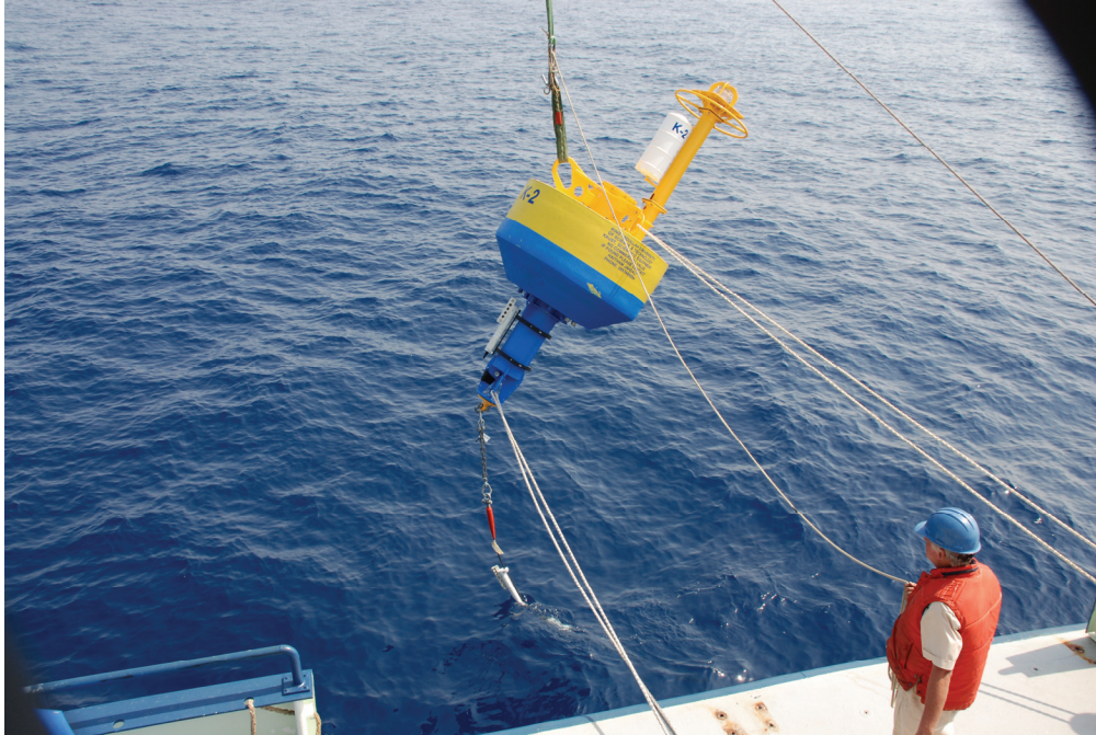
Figure IV-4: Deployment of mooring K2. A upper portion of the mooring line is visible (photograph courtesy of Susan Avery).
