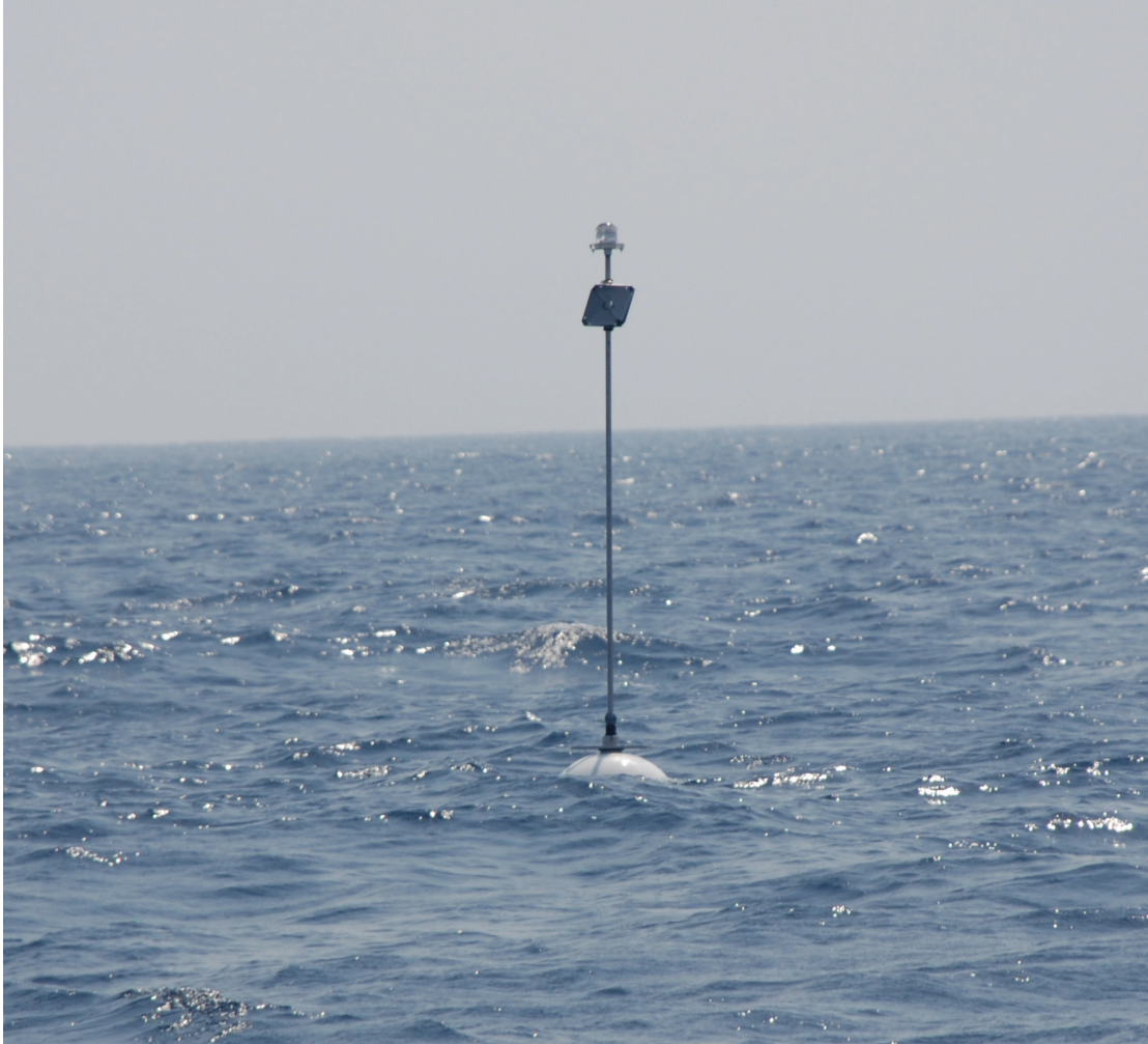
Figure IV-8: The surface buoy of the reef-edge mooring, showing the light and radar reflector at the top of the buoy mast.
