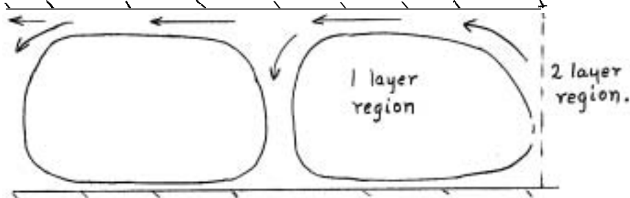
Fig.1 Plane sketch of observed boundary jet instability.
