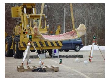
**Figure 1**: 3-D laser scanning of the mandible at the Woods Hole Oceanographic Institution (MA, USA) to determine the surface geometry.
