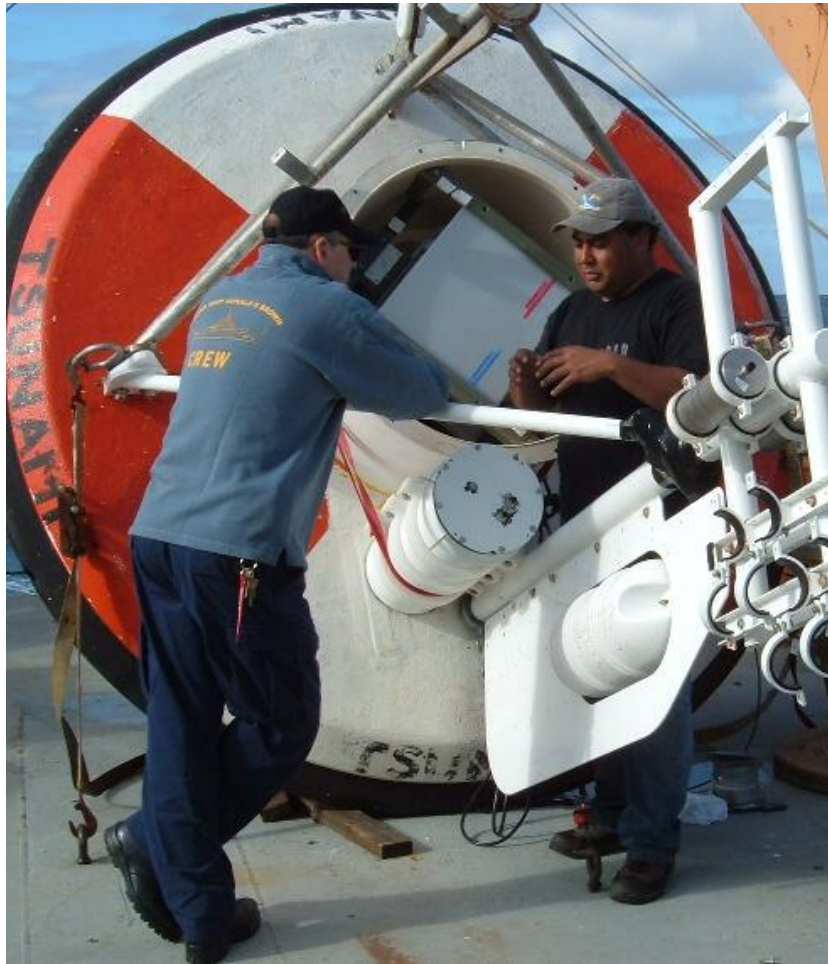
Fig 6-3: Working on the DART buoy
