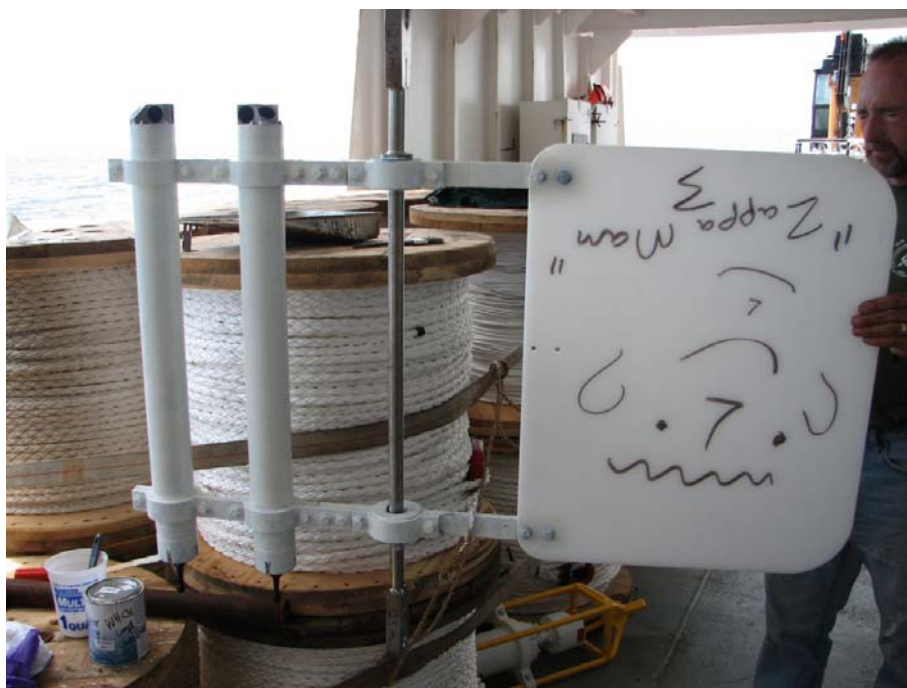
Figure 3-4: Picture of the vane system with two Aquadopp HR profilers. Note that the Aquadopp HR profilers and mounting brackets are painted with white anti-foul paint.
