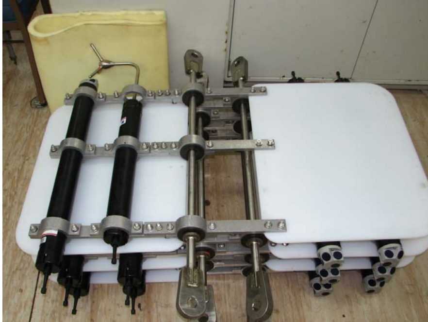
Figure 3-5: Picture of the vane system on Aquadopp HR profiler and one Vector ADV.
