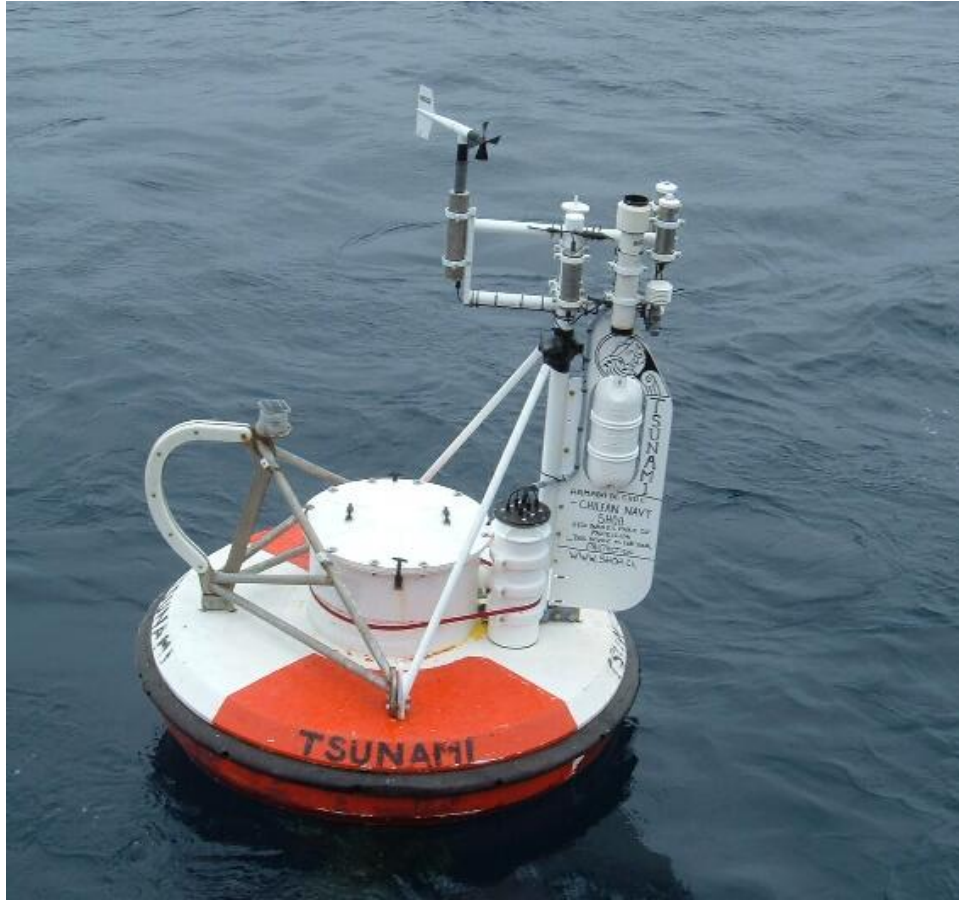
Figure 6-2: DART II surface mooring with a complete set of IMET sensors.
